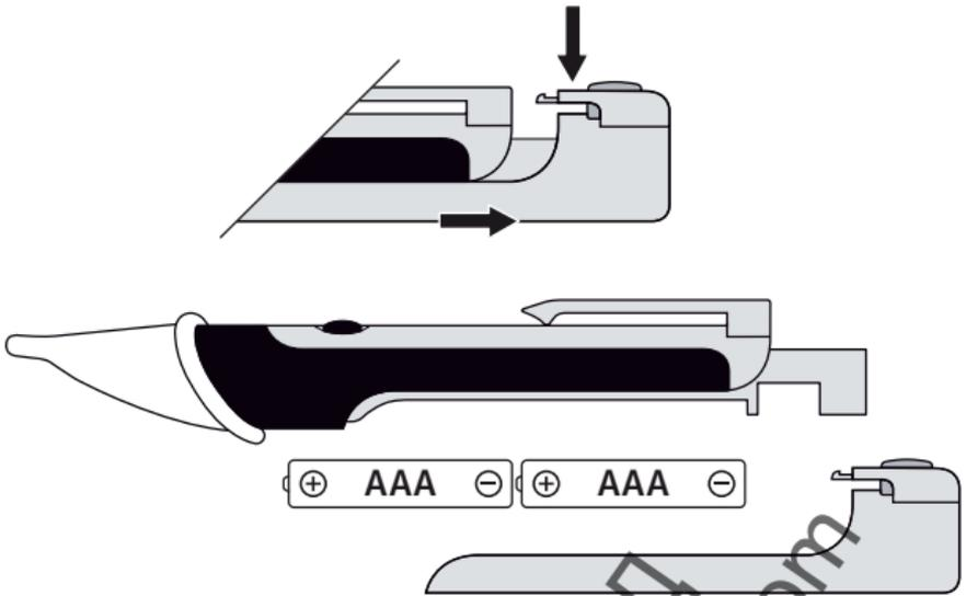
**!** The device is ready for use immediately once the batteries have been inserted. It does not have a separate ON/OFF switch and is therefore always active.
