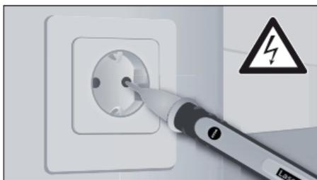
If voltage is present, the detector tip lights up and a signal sounds.
