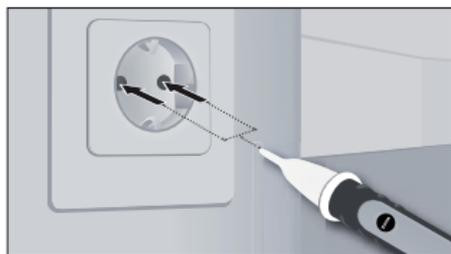
Position the detector tip in the area to be tested (e.g. cable, socket. etc.).
